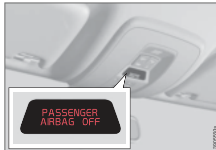
Indication in roof console
